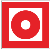
Pic. 294 Brandmelder manueel
